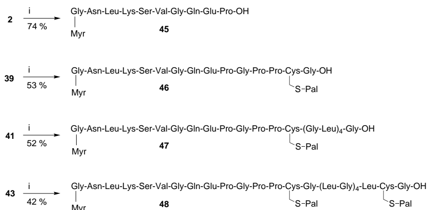
Scheme 7. Unmasking of the lipidated fragments 2 , 39 , 41 , and 43 . i) \text{CF}_3\text{COOH}/\text{ethanedithiol}/\text{H}_2\text{O} 95:2.5:2.5 (v/v/v).
